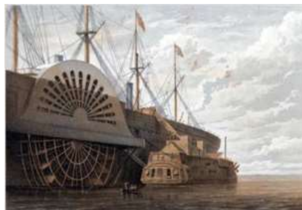
The old frigate Iris with her freight of cable alongside the Great Eastern at Sheerness. The cable passed from the hulk to the Great Eastern .
